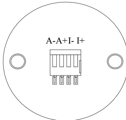
If the axle is kitted out of a plug (LUMBERG), connectors are marked as following :
