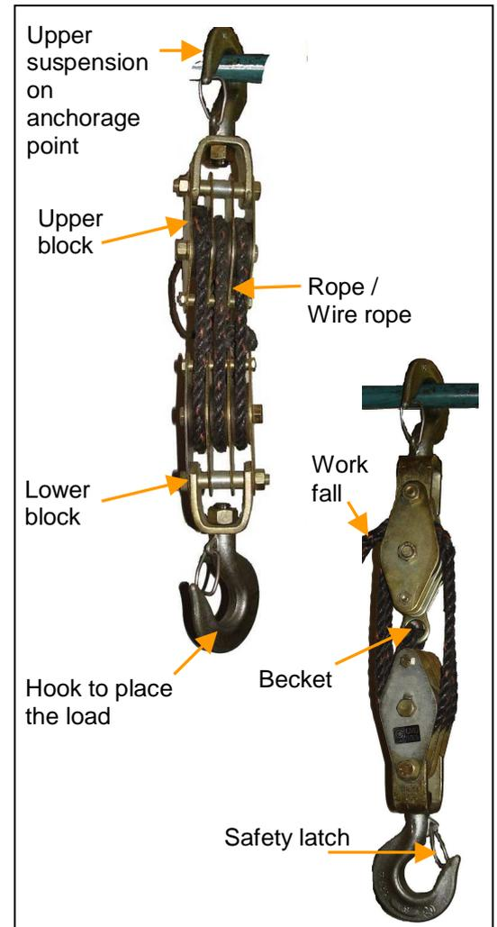
*Mechanical resistance of the upper block's anchorage point must at least correspond to the WLL of the block's upper suspension :*
